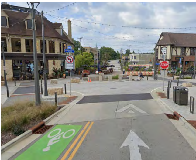
Example of a main street crossing and improved pedestrian experience with colored brick paver crosswalks and brick paver intersection. Image: Google Earth
